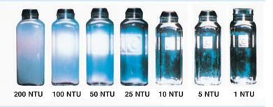
A few examples of turbidity expressed as Nephelometric Turbidity Units. The Filtr-Cleer process of filtration makes possible the reduction of the water turbidity to below 4 NTU (0.4 NTU for OFSY).
